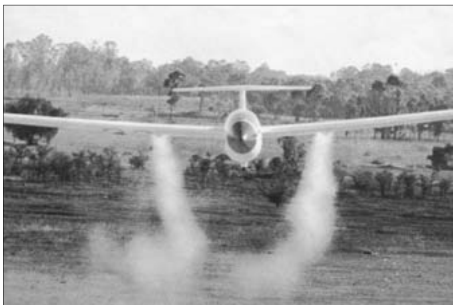
Cirrus piloted by Ted Pearson coming over the finishing line after task, dumping water prior to landing
