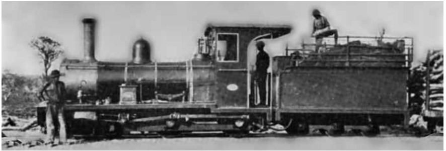
One of the Ex-Beira Railway locomotives referred to in the text. This was taken before a spark arrester was fitted, and the loco also has its original 6-wheeled tender. Shown clearly is the semi-elliptic leaf spring exposed above the leading driving wheel. Ex-Beira Railway locomotive crossing a bridge in the Rhodesdale Estate. Note the spark arrester on the chimney. Also shown is the ex-Beira Railway 4-wheeled coach.
