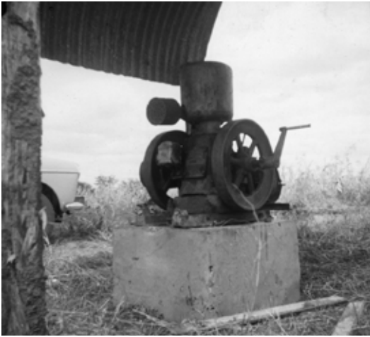
1927 Lister pump engine, used for pumping water from the Umsweswe River. It is still in use on Pat Conway's farm, near Gatooma.
