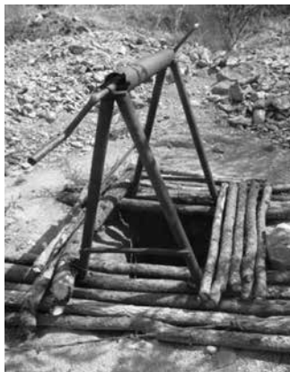
A windlass commonly used by artisanal gold miners above a shaft just below Fort Hill
