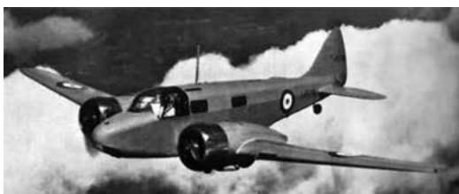
The Oxford Advanced Trainer (nicknamed the ‘Ox-box’) had dual controls and was used to train pilots, navigators, bomb aimers, gunners and radio operators.
