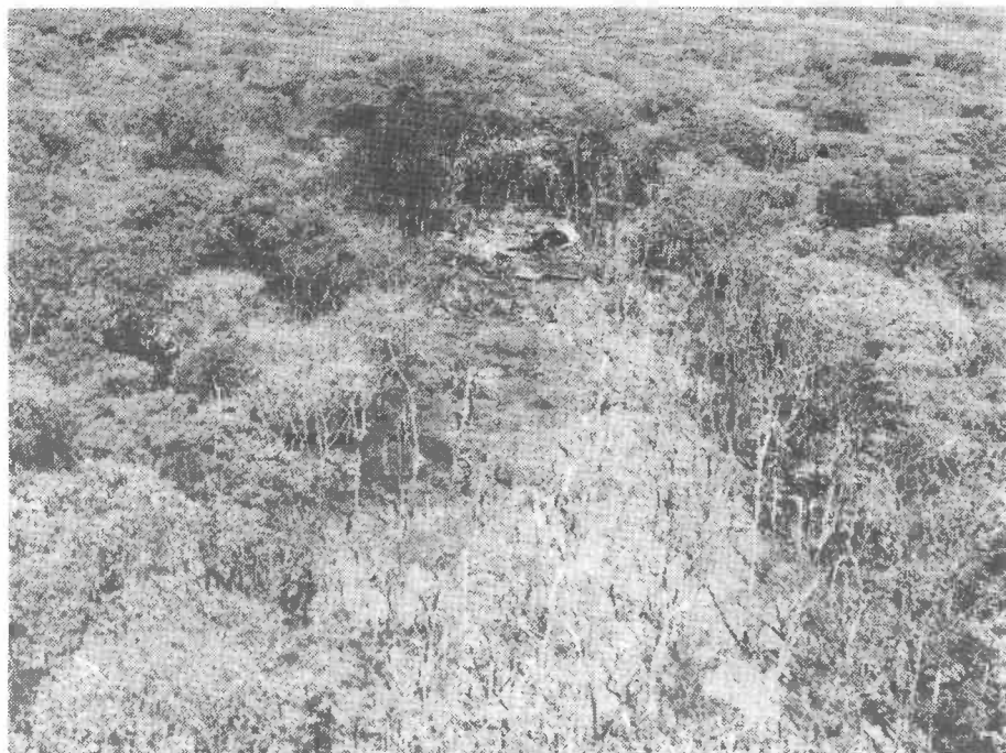
View of the DC6 approach path showing swathe cut in the trees indicating a normal angle of descent and lateral stability of the aircraft before impact
