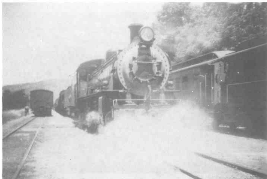
A Rhodesia Railways 12th Class 4-8-2 puts up steam on the line through Bechuanaland (Phil Killin)
