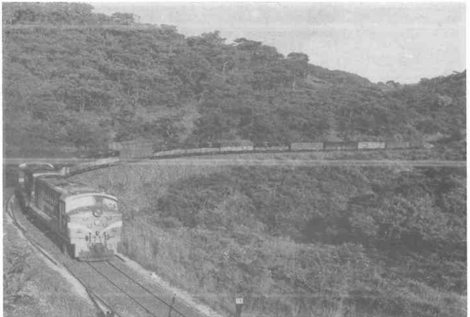
Class DE 3s in tandem working the most difficult section of the R.R. — Machipanda-Umtali. Note the speed limit on this sharp curve is 15 mph. (G. Pattison)
