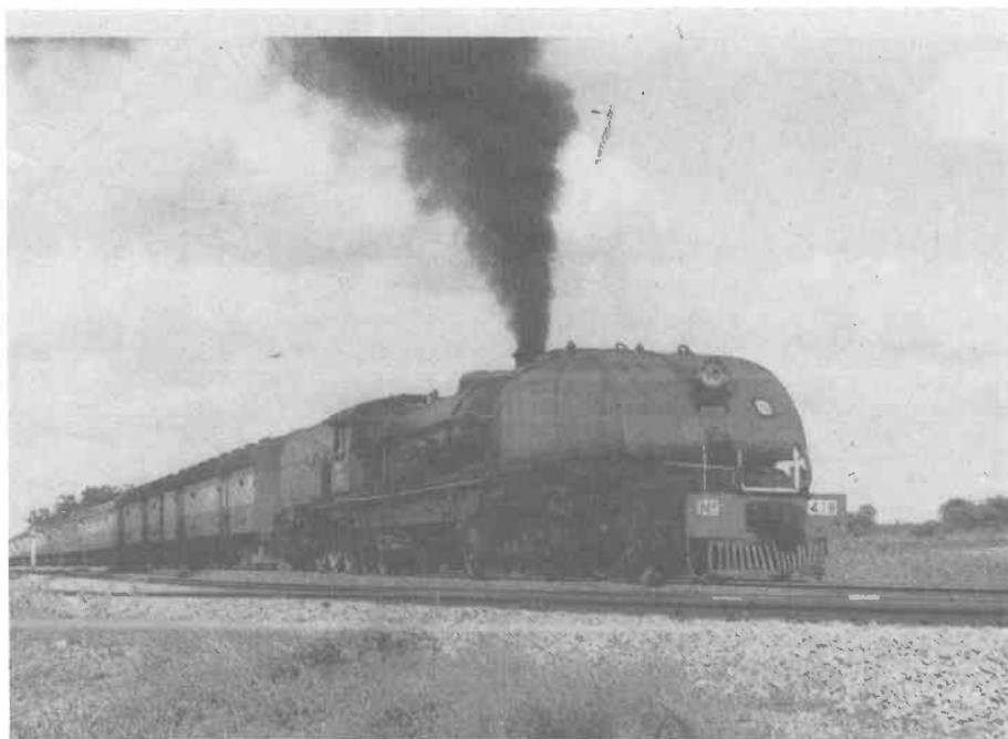
The Beyer, Peacock 15th Class Garratts were popular steam locomotives on the railway through Bechuanaland/Botswana from 1963 and reappeared from Bulawayo–Plumtree in the late eighties (J. Batwell)
