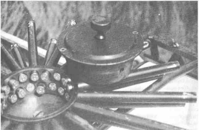
9. Spider anti-ambush weapon with breech-block removed to reveal the loaded cartridges. When travelling in convoy, barrels to the front and rear could be left unloaded
