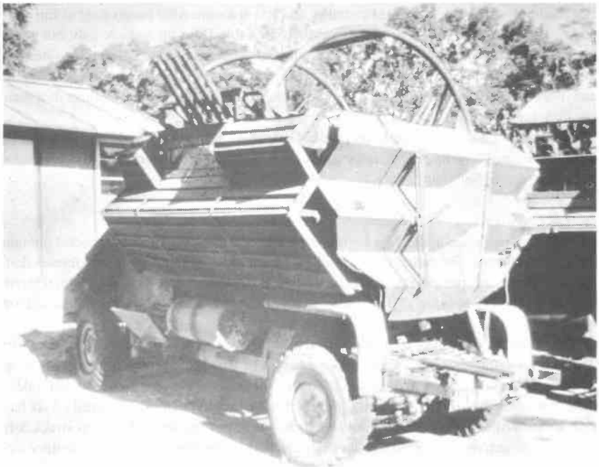
6. A "Kudu" mine and ambush protected vehicle fitted with a pair of multi-barrelled anti-ambush weapons. These are believed to be 5-barrelled versions of the Persuader shotgun which discharged on gravitational fall of the barrels. Note also the electrically fired, twin-barrelled weapon mounted at the rear of the vehicle
