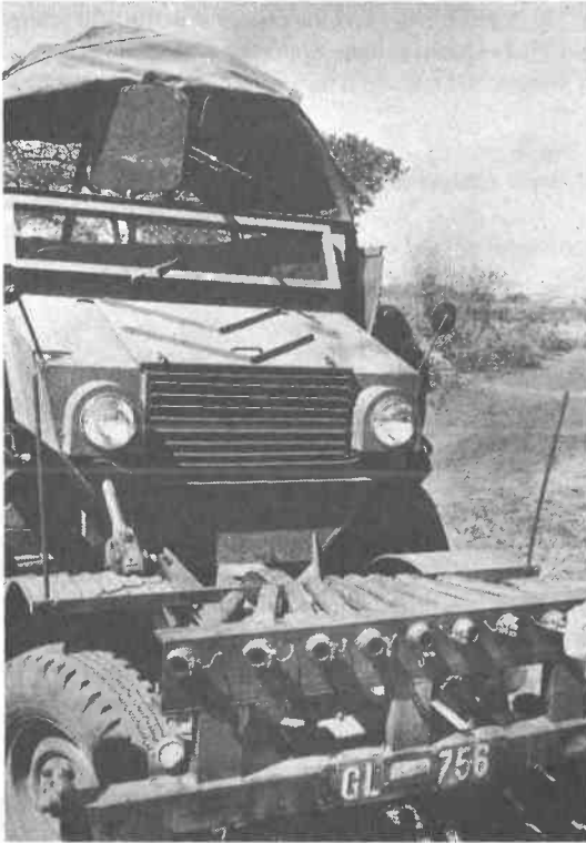
14. A forward mounted battery of the devastating Holland-Hail Organ, fitted to a “Cougar” mine and ambush protected vehicle. (The Sunday Mail)
