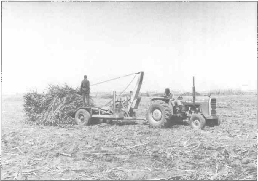
A six tonne bundle of sugarcane being loaded on to a Perry trailer
