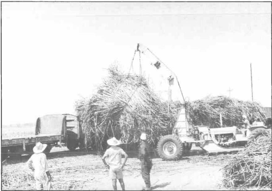
Hydraulic crane loading bundle on to train wagon
