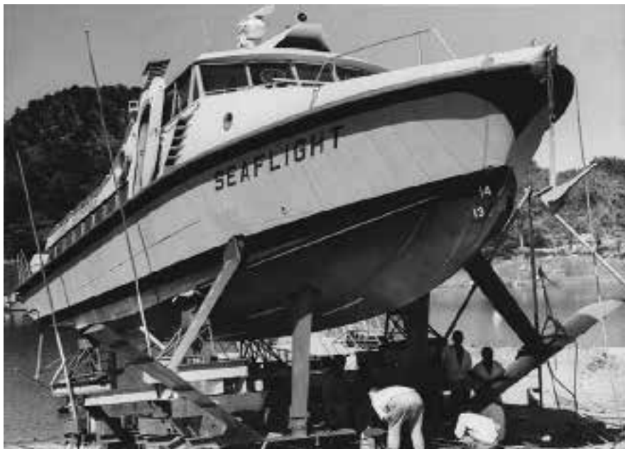
The final task—the foils being fitted, prior to the trial run on 7th May, 1972, when Seaflight would be skimming Rhodesian waters for the first time.
